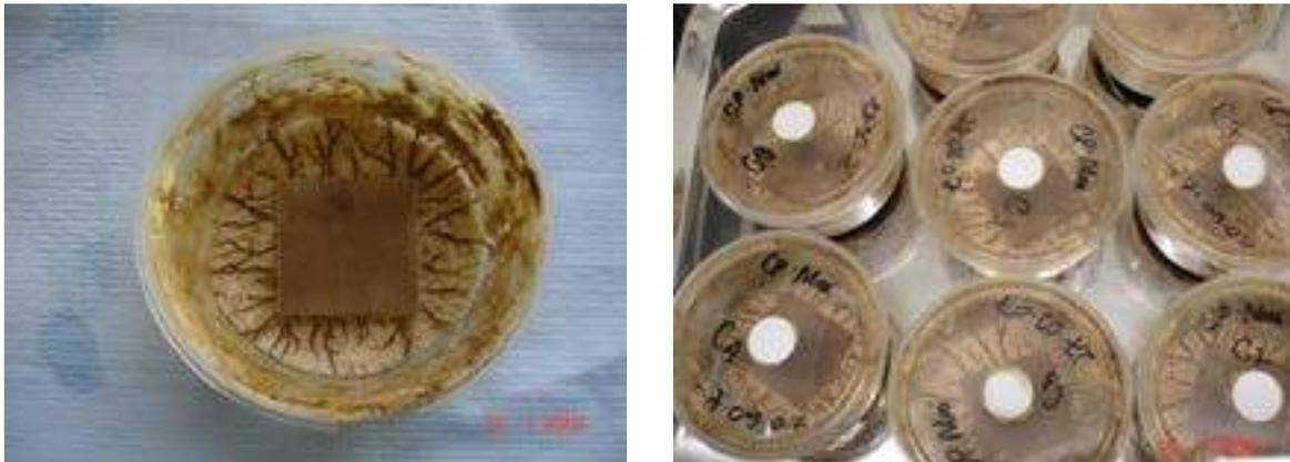
**Figure 1.** Plywood specimens after 16 weeks of incubation with *C. puteana*
